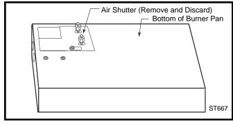
Fig. 18 Remove air shutter and discard.
